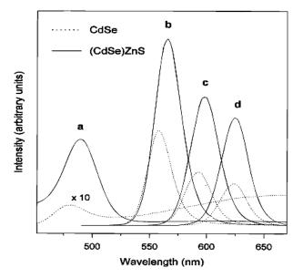
Fig. 3. Photoluminescence spectra for bare CdSe QDs (dashed lines) and CdSe/ZnS core/shell QDs (solid lines) [21].
