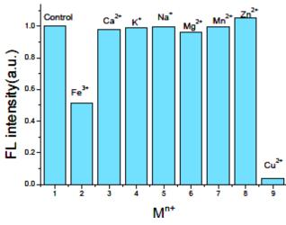
Fig. 9. Effect of biologically relevant ions on the fluorescence of BSA-QDs: concentration of  $Cu^{2+}$ :  $10^{-6}$  M; for others:  $5 \times 10^{-4}$  M [145].
