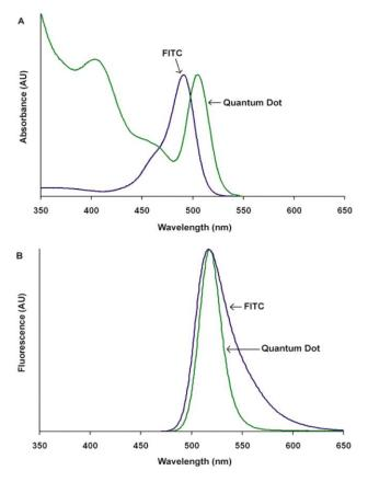
Fig. 5. Comparison of absorption spectra (A) and emission spectra (B) of QDs and fluorescein isothiocyanate organic dye (FITC) [18].
