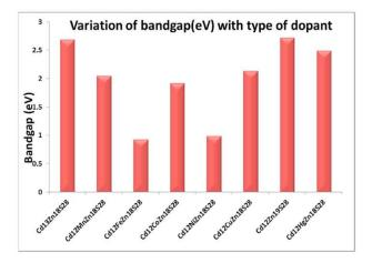
Fig. 4. Variation of the band gap of CdS/ZnS core/shell QD on doping with various transition metal ions.
