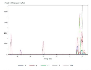
Fig. 6. Partial density of states (PDOS) plot for the undoped CdS/ZnS core/ shell QDs.
