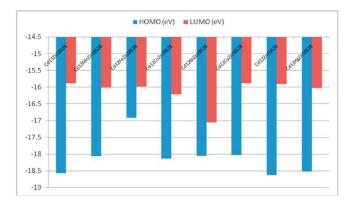
Fig. 5. Variation of HOMO and LUMO energy levels of CdS/ZnS core/shell QD on doping with the transition metal ions.
