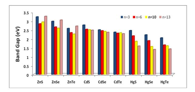
Fig. 3 Variation of the band gap (eV) for II-VI nanoclusters as a function of cluster size
