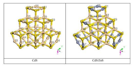
Fig. 2. Optimized structures of bare CdS and CdS/ZnS core/shell QDs. Bluish Gray- Zinc, Off-white- Cadmium, Yellow- Sulfur. (For interpretation of the references to colour in this figure legend, the reader is referred to the Web version of this article.)
