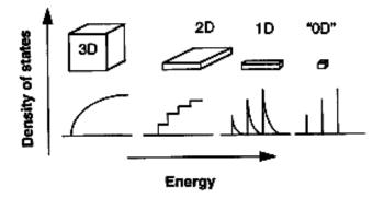
Fig. 1. Illustration of density of states in semiconductors as a function of dimension [19].
