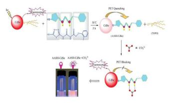
Fig. 11. Synthesis procedures of AASH functionalized CdSe QDs and a possible model for carbonate recognition [197].
