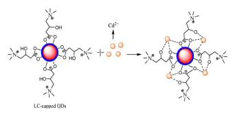
Fig. 10. Schematic illustration of interaction of LC-CdSe/ZnS with  $Cd^{2+}$  ions [164].
