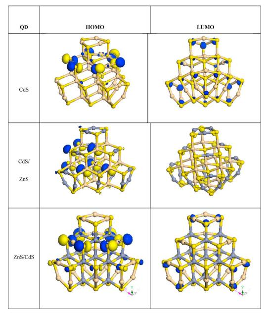
Fig. 3. HOMO-LUMO plots for bare CdS hexa-cationically charged QDs,CdS/ZnS and ZnS/CdScore/shell QDsBluish Gray-Zinc, Off-white-Cadmium, Yellow-Sulfur. (For interpretation of the references to colour in this figure legend, the reader is referred to the Web version of this article.)
